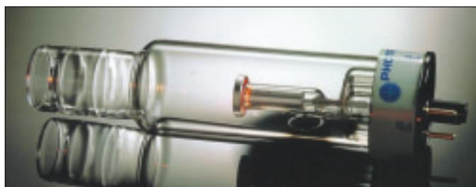
Figure 1. Photo of single-cathode multi-element lamp
