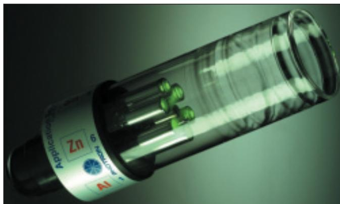
Figure 2. Photo of six-cathode lamp
